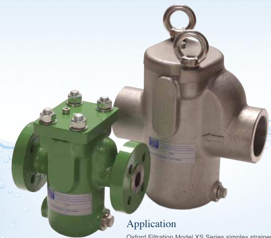
Oxford Filtration Model XS Series simplex strainers provide a simple cost-effective way to separate particle impurities from fluid flow systems. Simplex models described in this brochure are designed for applications where temporary interruption of a batch process can be permitted for basket cleaning. Where continuous, uninterrupted flow is required, our duplex strainers or self cleaning filters described in other brochures should be used. All strainers are individually pressure tested.
